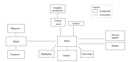
Figure 4: TFXlipse architecture shown as a component view
