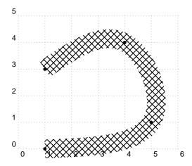
The \thickBspline macro works as expected in the closed (periodic) case, taking advantage of automatic incrementing of the nodecount. Note that \thickBspline interprets thickness as visual, unaffected by possible differences between xunit and yunit.
