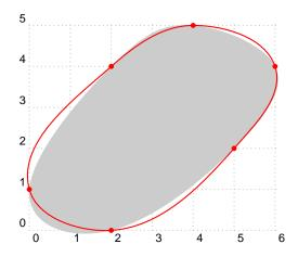
A B-spline curve can in many cases provide a good function interpolation mechanism, but the result is not guaranteed to be the graph of a function.
