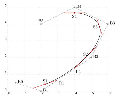
2.1. **Bézier curves as B-spline curves.** Consider a Bézier curve  $\mathscr C$  with control points  $S_1$ ,  $C_1$ ,  $C_2$ ,  $S_2$ . To identify  $\mathscr C$  as a B-spline curve of the type discussed above, consider the problem of finding the B-spline control points  $B_0$ ,  $B_1$ ,  $B_2$ ,  $B_3$  for which \psBsplineE yields  $\mathscr C$ . This is a simple problem in linear algebra whose solution is:
