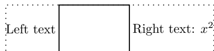
Figure 44: The macro s_box sets string dimensions automatically when processed twice. If two or more arguments are given to s_box , they are passed through sprintf . The dots show the figure bounding box.
